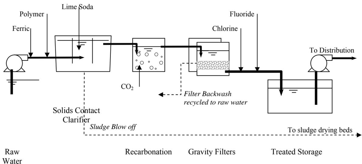
Figure 2 is a schematic of the existing process.
